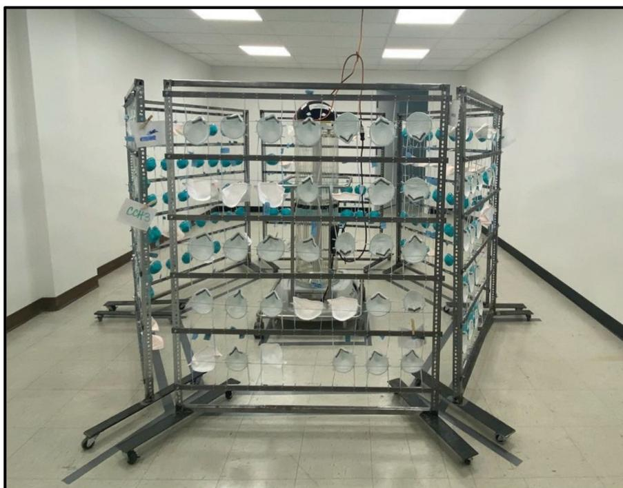
Figures G & H: Trellis configuration in decontamination room
